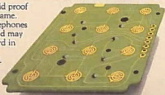
Long-life, non-corroding, gold-plated contacts.
