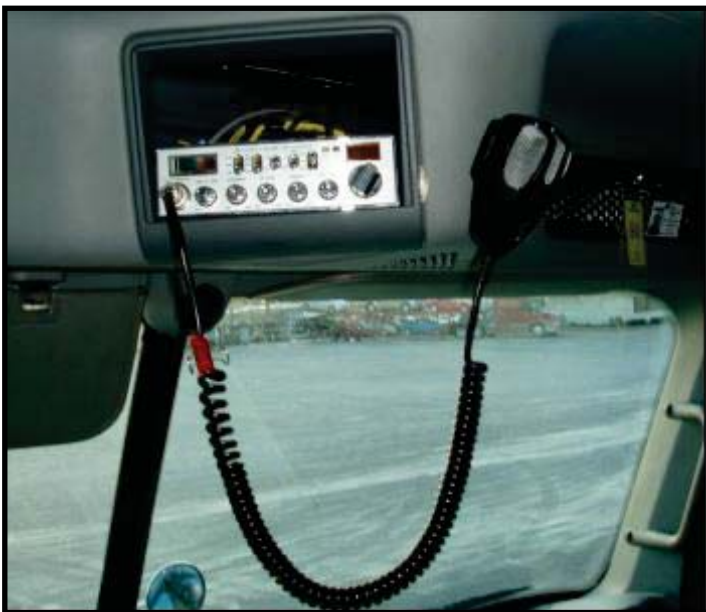
A Typical CB Installation
