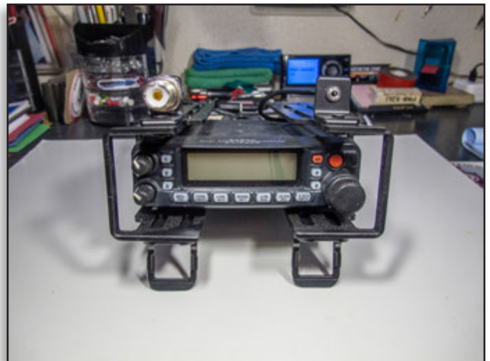
Figure 11: Addition of flip-down feet to elevate radio to a more comfortable operating position.
