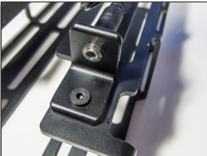
Figure 8: Speaker connector mounted to the rails
