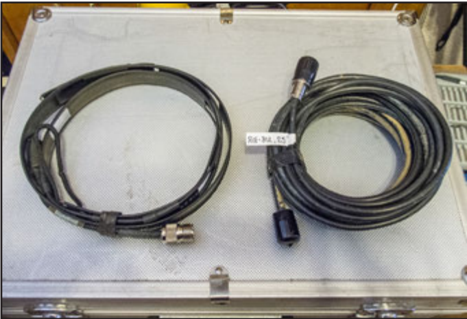
Figure 14: N9TAX dual-band roll-up J-Pole antenna (L) and 25 ft length of RG-8U coax (R)
