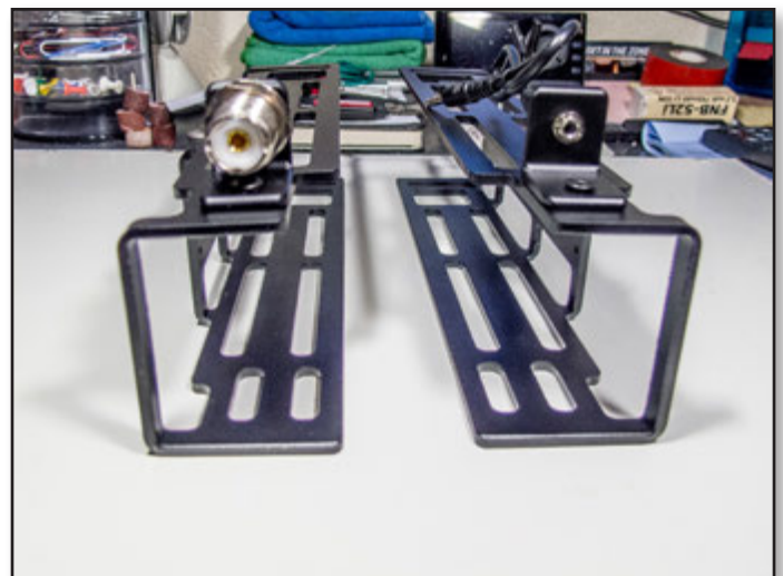
Figure 6: ARMOLOQ rails with SO-239 and speaker connectors mounted
