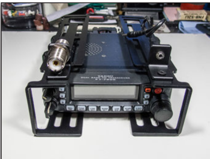
Figure 9: FT-7900R radio with rails attached.
