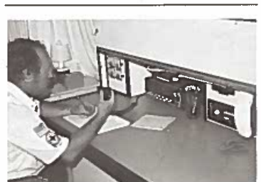
SAN ANGELO, Tex.—The San Angelo REACT Association (Team #3387) has a new $1,500 base station console built entirely by the members. Constructed with plywood laminated with orange and white Formica, the unit is designed to accommodate two operators. In case of a power failure, the console switches automatically from AC to DC power through a relay system. Meters measure both AC and DC power output. The console may be closed and locked when not in use and can be easily disassembled and transported to another location if necessary.
